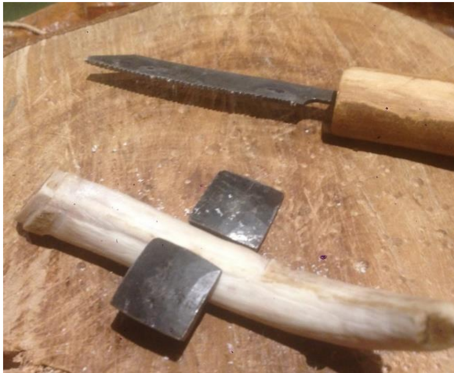
Figure 11: Using the rasp saw to further define the spine
