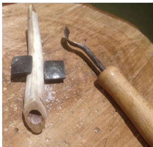
Figure 10: Marking out the spine ridge with a gouge
